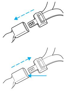
2. To unfasten, push the release button and remove the tongue from the buckle.
